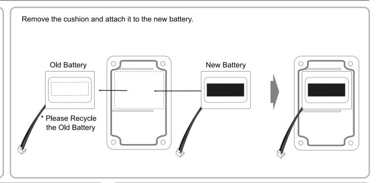
Reinstall new battery and reconnect the connector. Be careful to keep the wire away from transformer.
