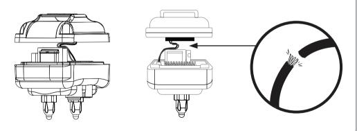
Be mindful not to pinch the wire as seen in the figure below or broken wire may occur.
